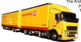
The first of 11 trailers went on the road in October 2012. Craig has had 5 x 6 axle curtain-side B-trains and 6 x 5 axle curtain-side full trailers built by Fruehauf Trailers in Fielding using NZH Gigant DKH2 19.5 disc axle combined with Gigant's FB70 air bag suspension. The axles are fitted with the well known Wabco PAN 19 calliper, an SKF cartridge grease filled bearing assembly, and fully enclosed EBS pole wheels and sensors.
