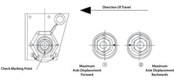
Using an open ended AF60 spanner, and making sure the spring bolt is tightened to at least 200Nm turn the ecdentric bushes on both sides of the hanger bracket to adjust the axle track. Using the Gigant adjustment tool part number 00311045 makes this job easier.
